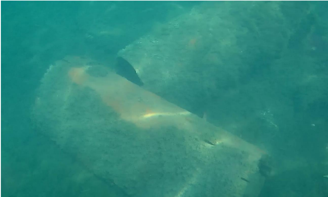
Figure 10: 2 pieces of steel pipe, 1 m long – 500 mm diameter, left by Subsea Tech 5 years ago for ROV pilot training purposes.
