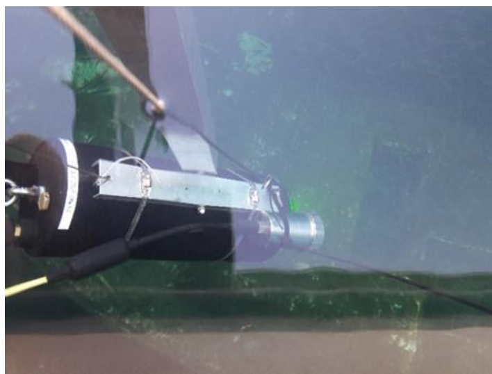
Figure 27: Utofia and conventional cameras hung alongside the quay
