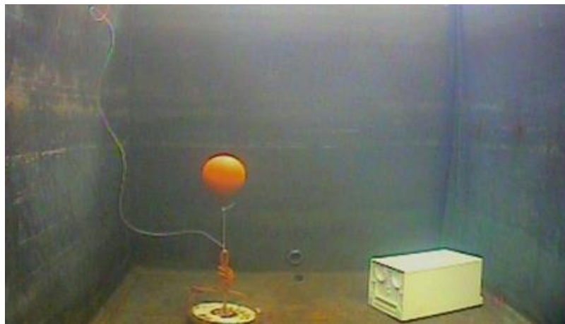
Figure 24: The two targets used for the Utofia tests: orange float and white plastic box
