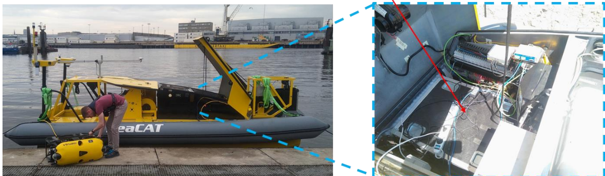
Figure 8: SeaCat electronics compartment
