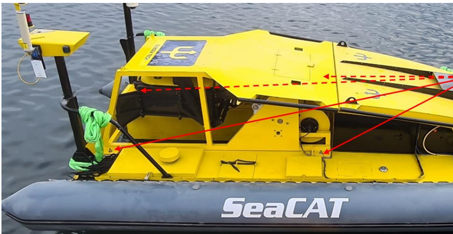
Figure 17: cROV LARS mechanical mounting
