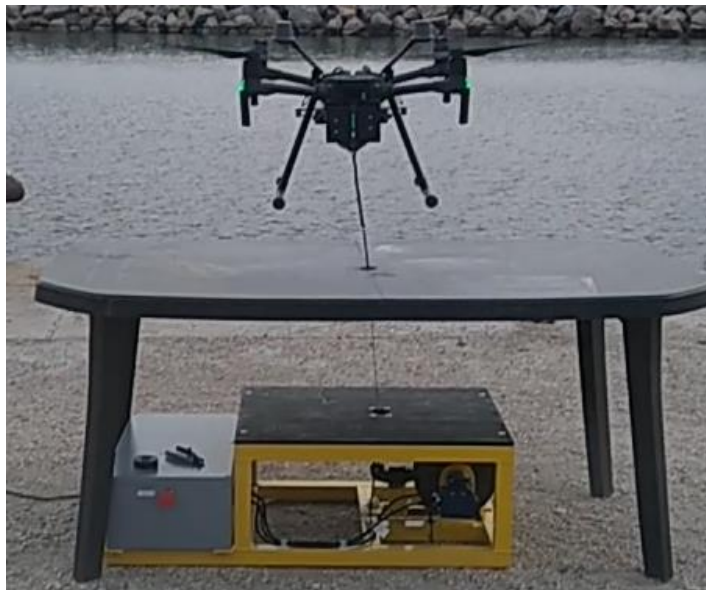
Figure 19: Tethered UAV launched from its LARS
