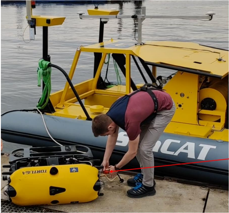
Figure 18: cROV LARS connection to the ROV
