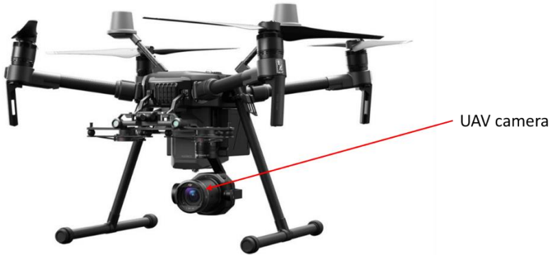
Figure 2 - UAV, DJI Matrice 210 V2, camera
