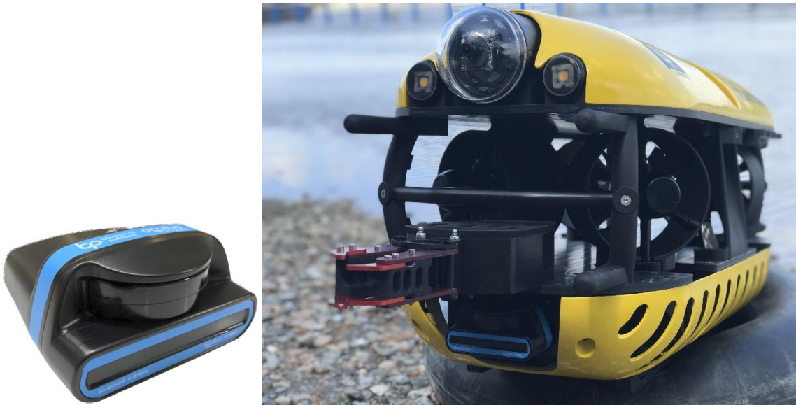
Figure 3: Blueprint Oculus 750d sonar mounted on Tortuga ROV
