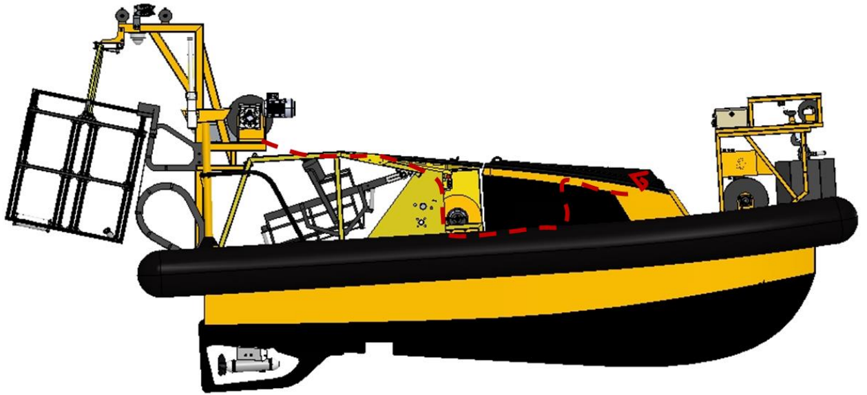
Figure 24: Basket LARS power/Ethernet wiring
