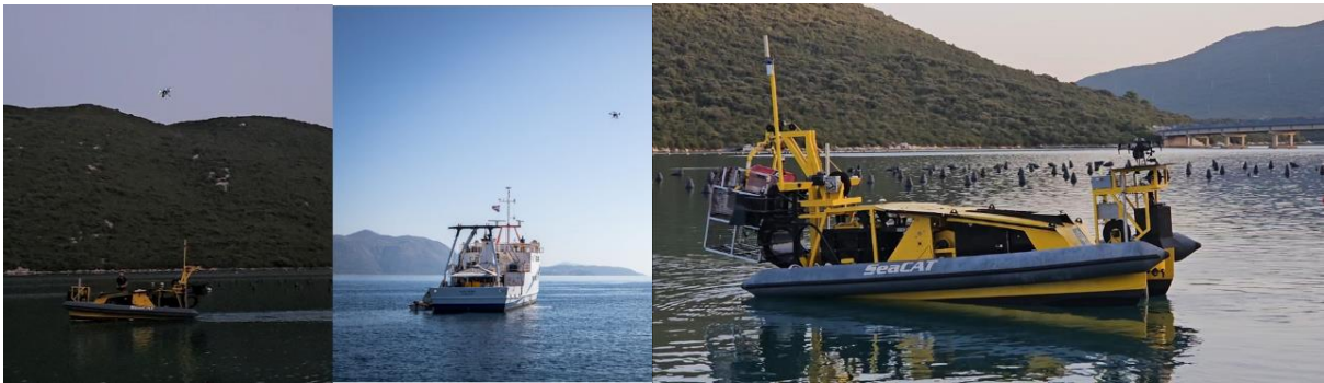
Figure 20. UAV in free flight and a tethered drone on a landing platform onboard of the SeaCat
