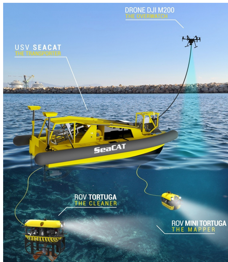
Figure 1: SeaClear concept. An unmanned surface vehicle acts as the hub of the system, an observation underwater vehicle maps the litter, and a collection underwater vehicle collects each piece of litter in turn, possibly also using a suction device to collect smaller litter. A UAV assists with detection and navigation surveillance.
